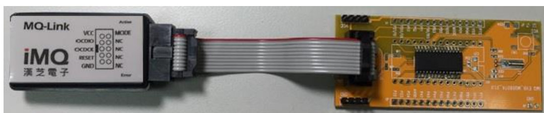
Figure 2.2 Connection between MQ-Link and EV Board (there is a product chip on the EV Board)
