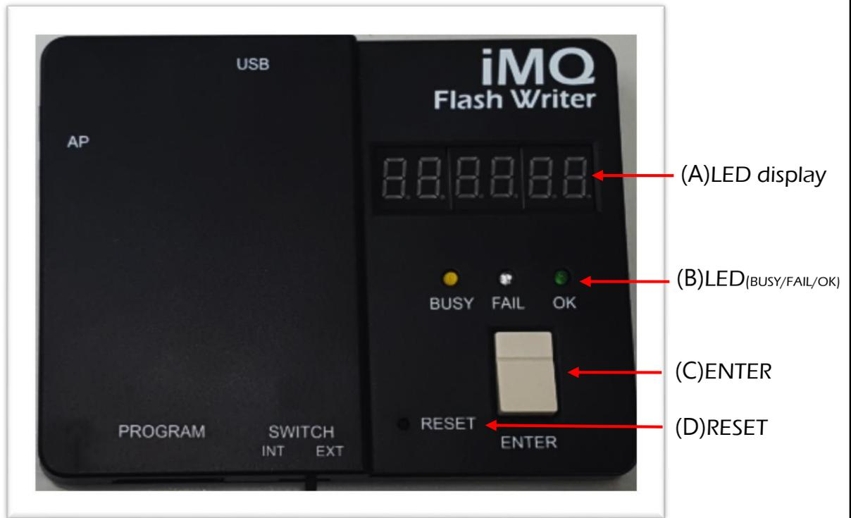
Figure 4- 1 Flash Writer Top View
