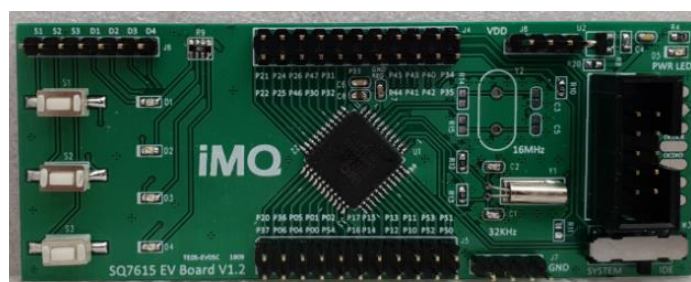
图2-2 EV Board 正面外观图(以SQ7615 EVB为例)
