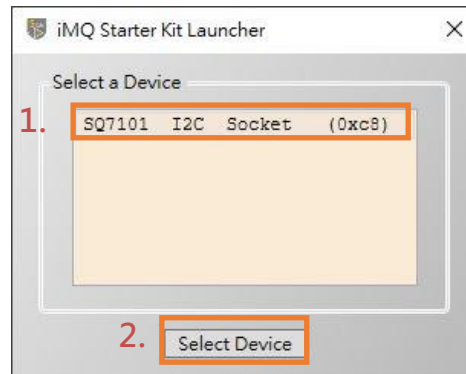
Figure 3.1 Using the Secure Starter Kit, and Socket is SQ7101 (I2C) device.
