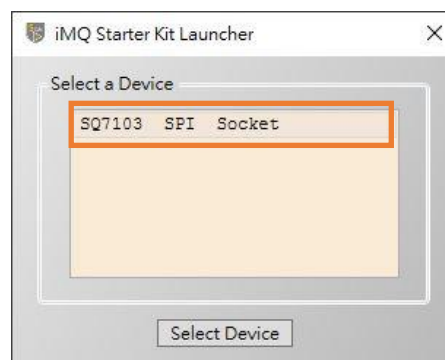
Figure 3.2 Using the Secure Starter Kit, and Socket is SQ7103 (SPI) device.
